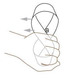
Step 7: In order to tighten the top screw you need to bend very gently the Apeiro until you have access to the top screw head. Compress, very gently, the bottom part of the Apeiro (see above) by holding it in your fist and squeezing. Tighten the top screw head only. The bottom screw does not need to be tightened.
