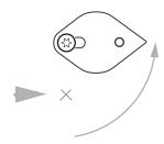
**Step 4**: Rotate the back plate in order to drill the bottom hole and insert the plastic plug in the wall.
