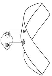
Step 6: Insert the Apeiro over the screw heads and press down until you feel a small "click". If in doupt, try to lift the Apeiro from the back plate. If it comes out easily then tighten the screws a bit more (as in step 5) and try again. If you can not put the Apeiro over the screw heads then make the gap (step 5) bigger and try again.
