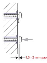
**Step 5**: Screw the bottom screw to the wall also. Do not tighten fully - allow 1,5 -2 mm gap on both screws so as to be able to insert the Apeiro over the screw heads
