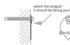
Step 2: Insert the plastic plug in the hole - screw the back plate to the wall using the top screw - do not tighten the screw!
